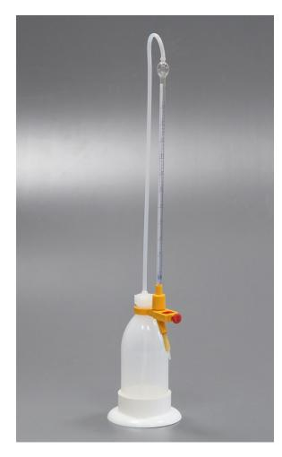
Method of Construction: Parts push together, they can be dis-assembled for cleaning
